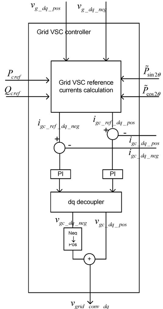
Fig. 10. Dual sequence current controller of grid VSC.
