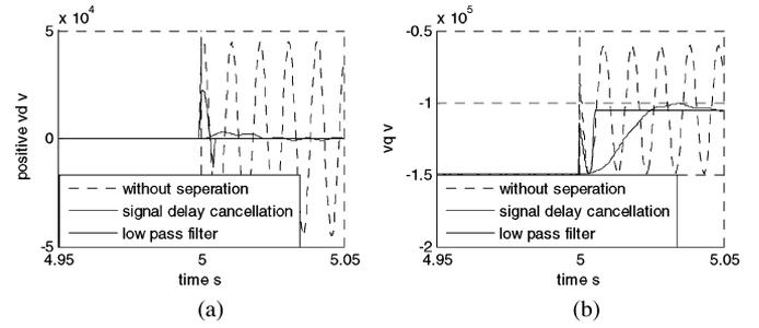
Fig. 8. Unbalanced voltages in positive  $dq$  reference frame with and without using the two separation methods (a)  $vd$  and (b)  $vq$ .
