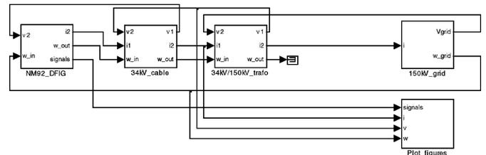
Fig. 3. Simulink model of DFIG system.
