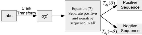
Fig. 7. Separate positive and negative sequences by “signal delay cancellation” method.
