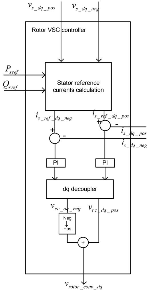
Fig. 9. Dual sequence current controller of rotor VSC.
